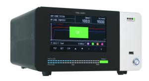
The T9731 - EN 14683 is specifically designed for measure the adequate air flow rate in complete adherence to the standard EN 14683.
